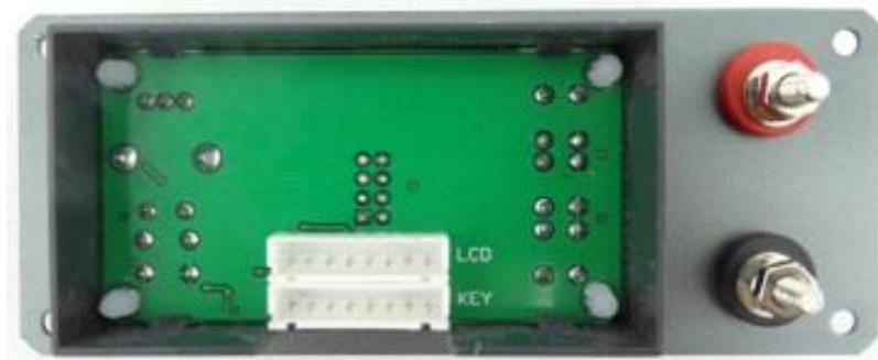
3.2.5 Install the output binding post, and use the output line with cold press connecting terminal to connect input (red is positive above, black is negative below), and screw it tightly
