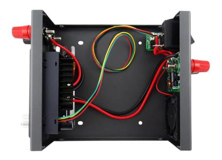
3.4 Extended application extension: you can put 10 pcs 18650 battery in series in the middle on housing to be input power supply. This will be a handheld mobile high-power dc stabilized voltage power supply
