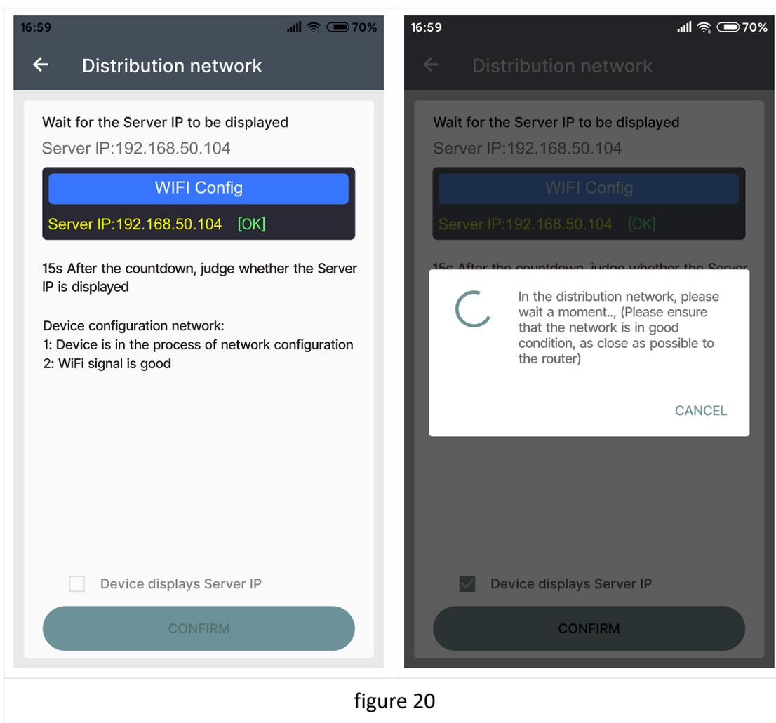
If the distribution network fails, please power off the module and re-operate in the same way (multiple networking failures you can watch the video and try to use the hotspot of the mobile phone to test). **If you use Huawei brand phone, please turn off the random MAC address function.**
